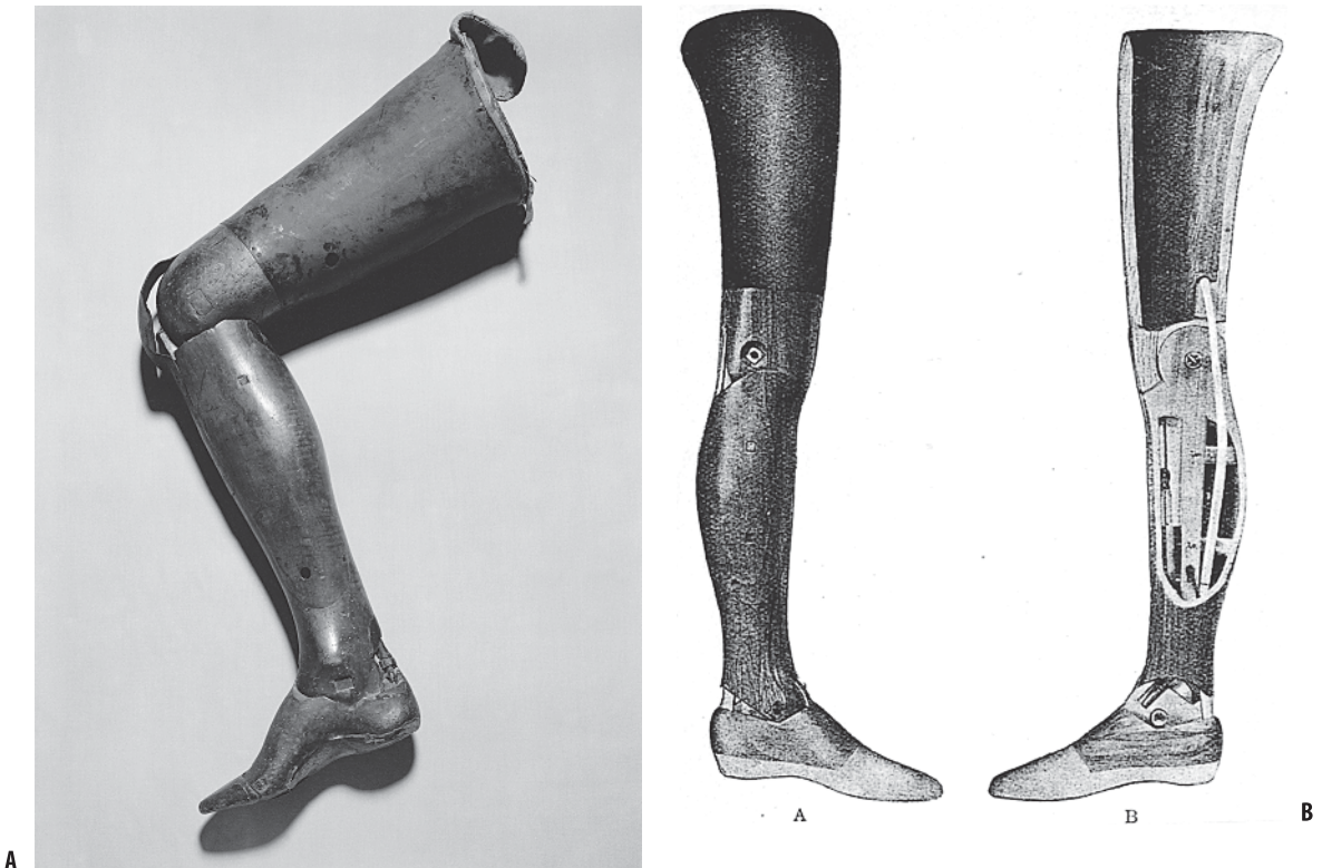
FIG. 13.5. a. Marquess of Anglesey’s leg made by Potts of London, c. 1820. This light limb in wood also coordinated ankle and knee movements, proving a successful solution for above-knee amputees over many years. This prosthesis is exhibited in Plas
