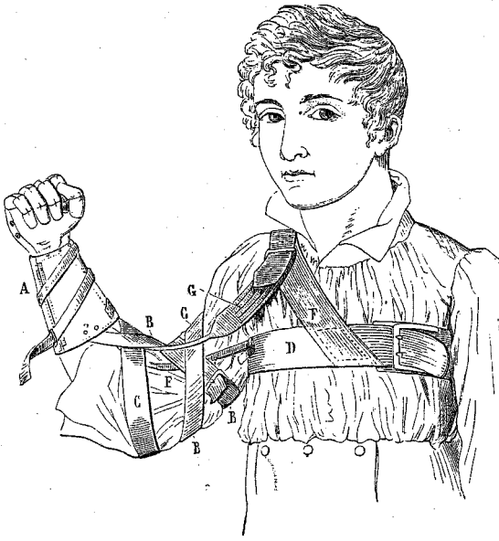
FIG. 13.6. Bailiff's prosthesis for forearm amputation, the first to utilise the trunk muscles to open an artificial hand otherwise kept closed by springs, 1818. (From Watson AB. A Treatise on Amputations of the Extremities and Their Complications . Philadelphia: Blakiston, 1885: fig. 159. 4 )
